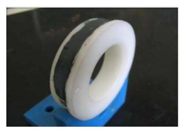
3. Insert the support into the differential with the oil hole at the bottom.
