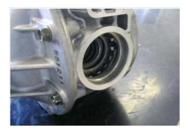
2. Apply oil resistant RTV sealant to the outer surface of the drive shaft support.
